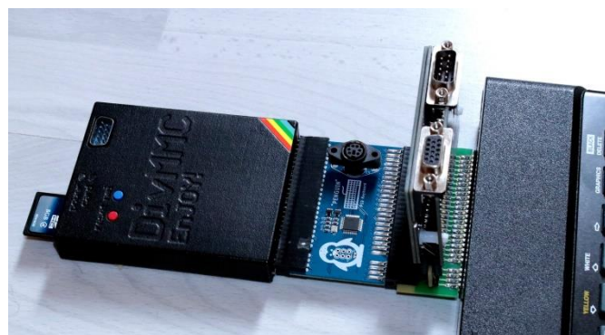
The PENGUIN together with the DIVMMC and the VGA JOY on a Y- adapter
